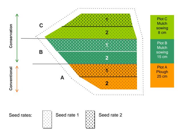
Initially, a stubble cultivation is carried out over all the plots with a compact disc harrow. Plot A is ploughed at a depth of 25 cm. In the min-till plots B and C, the soil tillage is carried out with a tine and disc combination cultivator in plot B at a depth of 15 cm following a pass with the compact disc harrow at a depth of 8 cm over both B and C.
