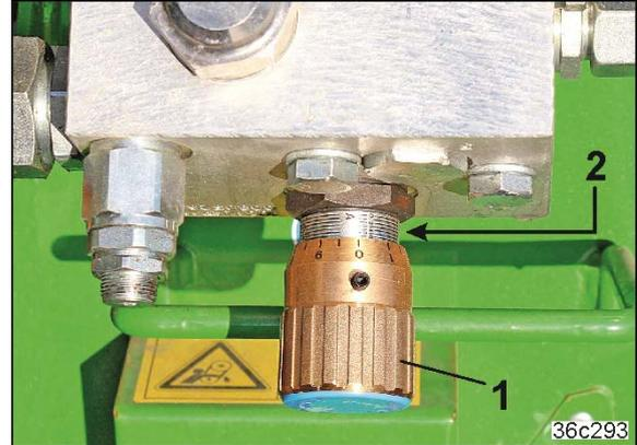
4. Set the blower fan to the required blower fan speed.
