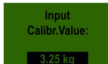
The theoretical seeding shaft speed is calculated from the initial data (working width and forward speed). If the calibrated seeding shaft speed deviates by more than 3%
