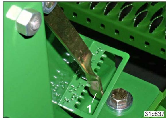
Adjusting the lever allows finer adjustment of the seed spread rate.
