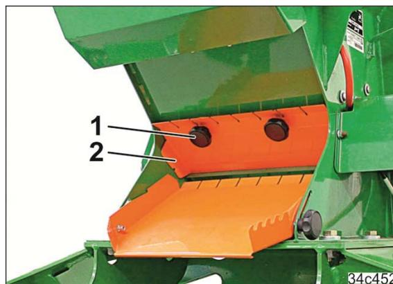
2. Release the star handle (1), push up the chute (2) and re-fasten.
