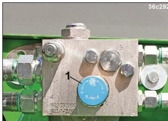
To ensure that the seeding shaft can only be switched on when the blower fan is running, the switch position of the blower fan is requested by a pressure sensor (1).
