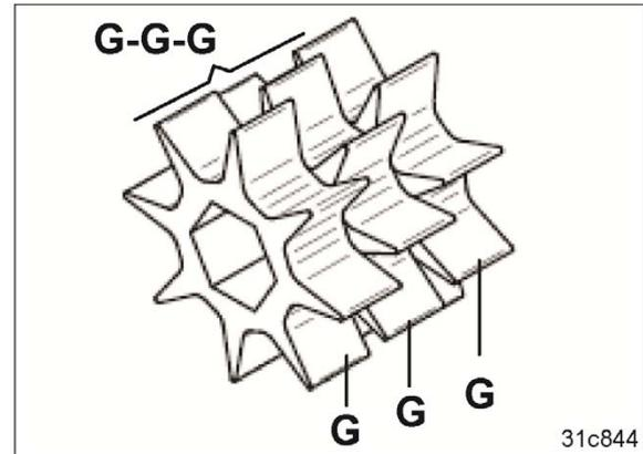
If it is necessary to exchange the seed metering wheels, the seeding shaft is pulled out of the metering unit. The seed metering wheels can be individually exchanged on the seeding shaft. It is more convenient to equip a second seeding shaft with the required seed metering wheels. Then only the seeding shafts need to be exchanged.
