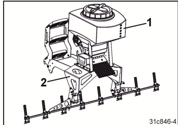
If you have purchased the GreenDrill (1) without an assembly set, it is considered as an incomplete implement. Without the assembly set, the GreenDrill is marked with a factory plate (see below) and an EC Declaration of Incorporation is included. The EC Declaration of Incorporation states that the product fulfills the relevant basic safety and health requirements of the EC Directive as well as the requirements of the EMC Directive.
