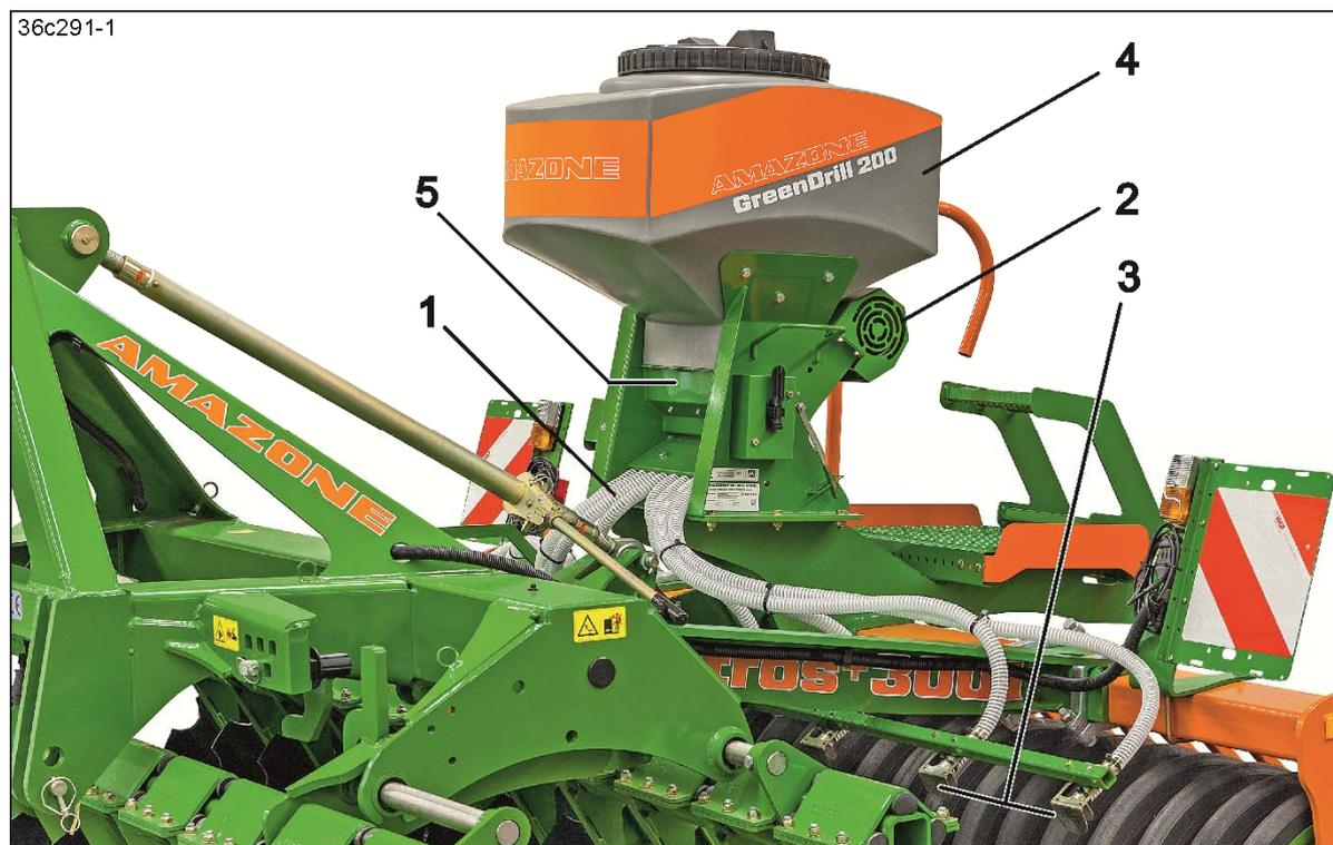
The GreenDrill is used for spreading catch crops and re-seeding grass.
