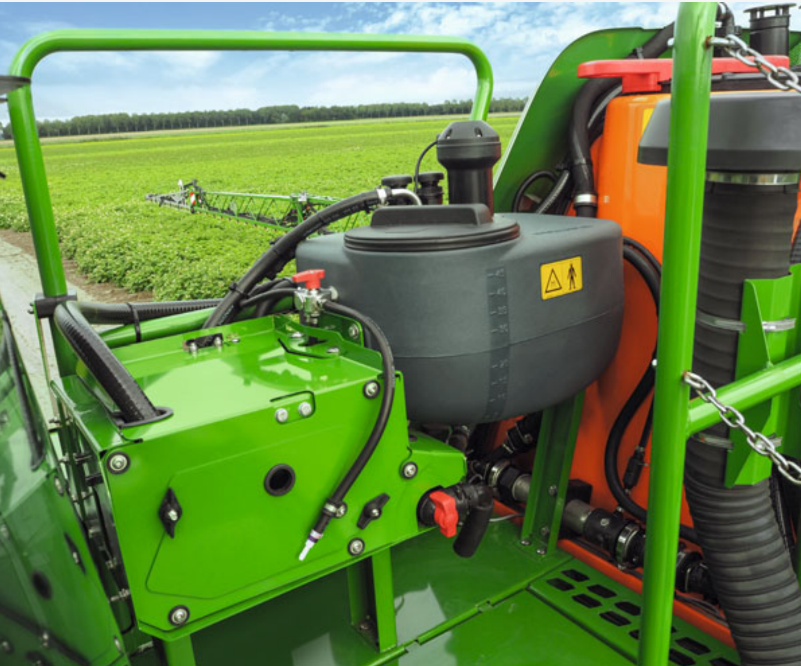
DirectInject on the Pantera 4504 between the cab and spray agent tank
