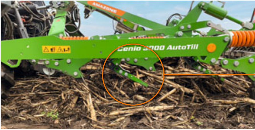
Blockage detection integrated in the tine element
