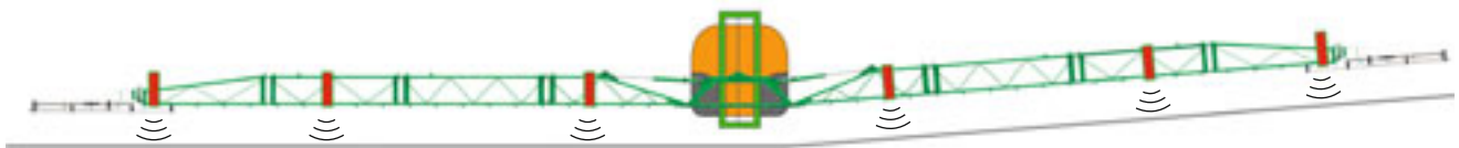
One-sided positive angling on the right (Flex-fold)
