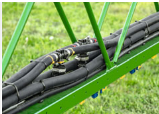
Injection points of the 2 spray lines into the liquid circuit
