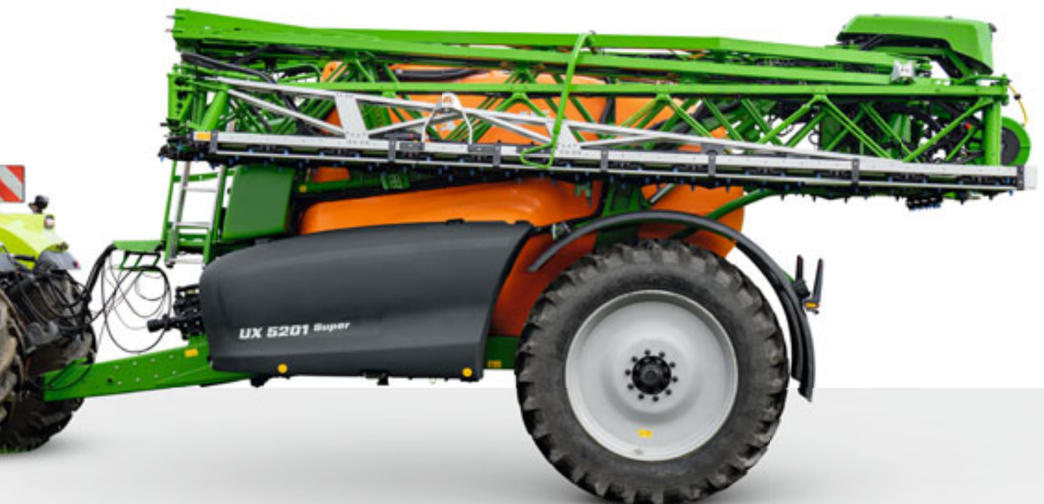
48 m wide Super-L3 boom – compact dimensions when folded for transport
