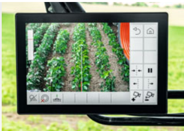
The camera system is operated via a high-resolution 10" terminal.
