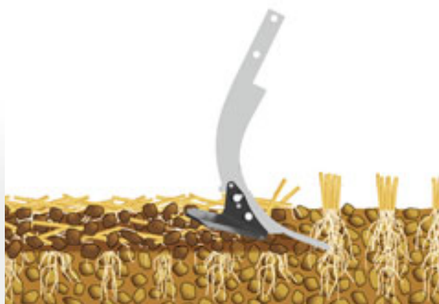
The steep angle of attack in Position 3 enhances the mixing of the organic matter in the soil.
