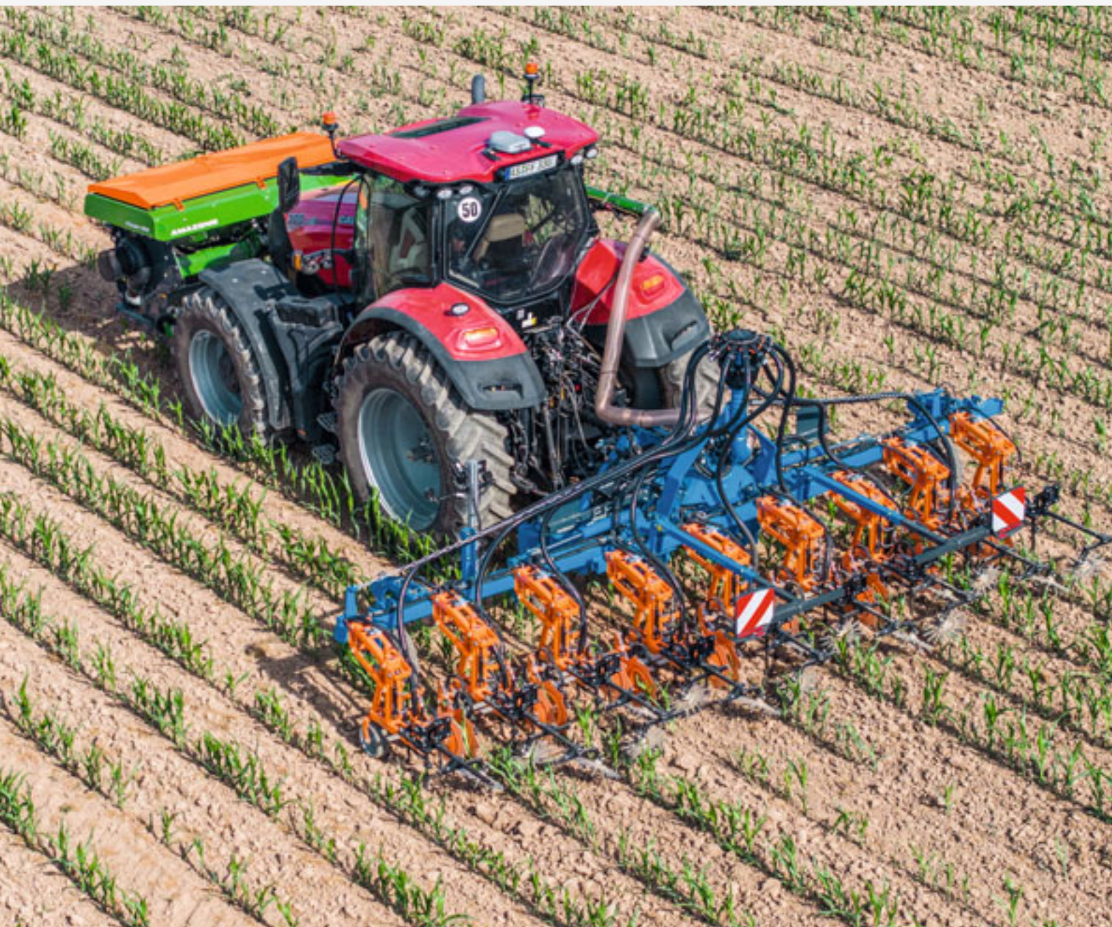
SCHMOTZER Venterra 2K hoe in combination with the AMAZONE FTender 1600 mounted front hopper for weed control and fertilisation in one pass.
