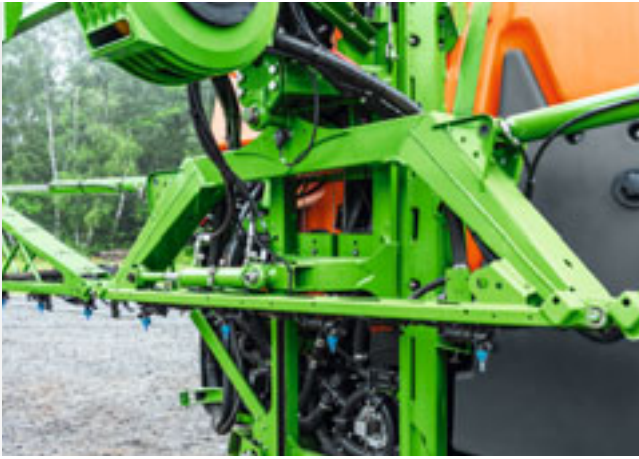
Fully automatic, active boom guidance via ContourControl
