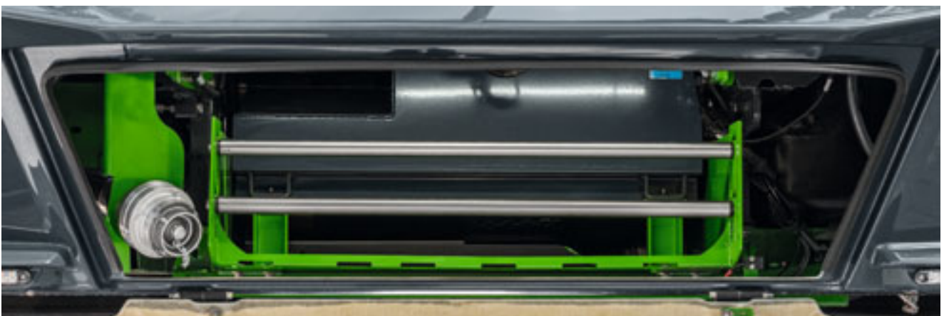
Illuminated storage compartment under the cab with bowser fill port and automatic fill stop
