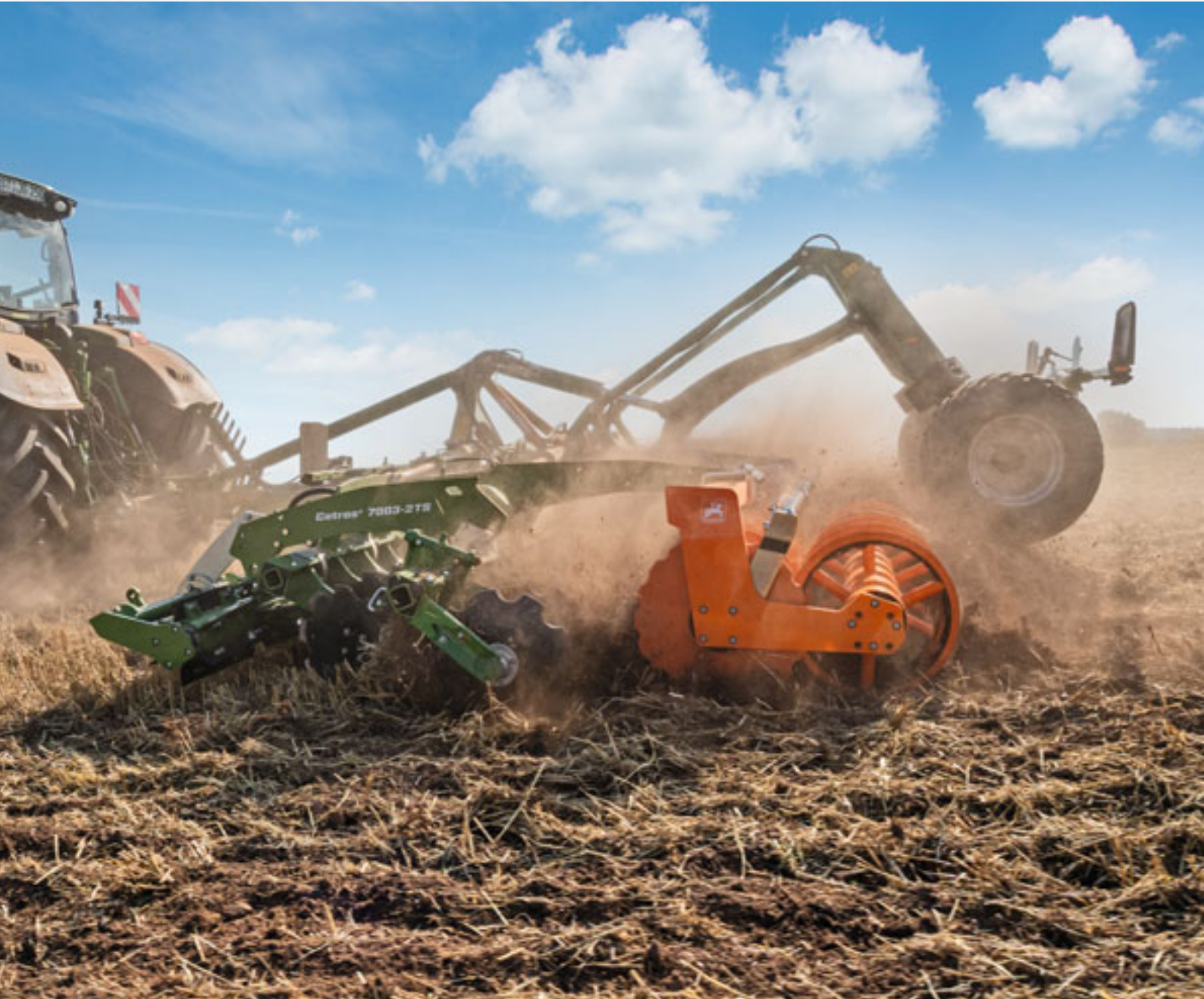
Catros + 7003-2TS with knife roller and double harrow
