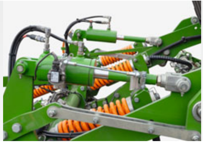
Distance measuring system for setting the working depth via the rear roller
