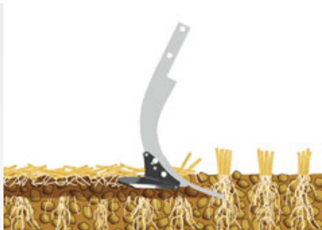
Optimum pull-in, thanks to the improved undercut of the point in Position 2, even in extremely dry soils.
