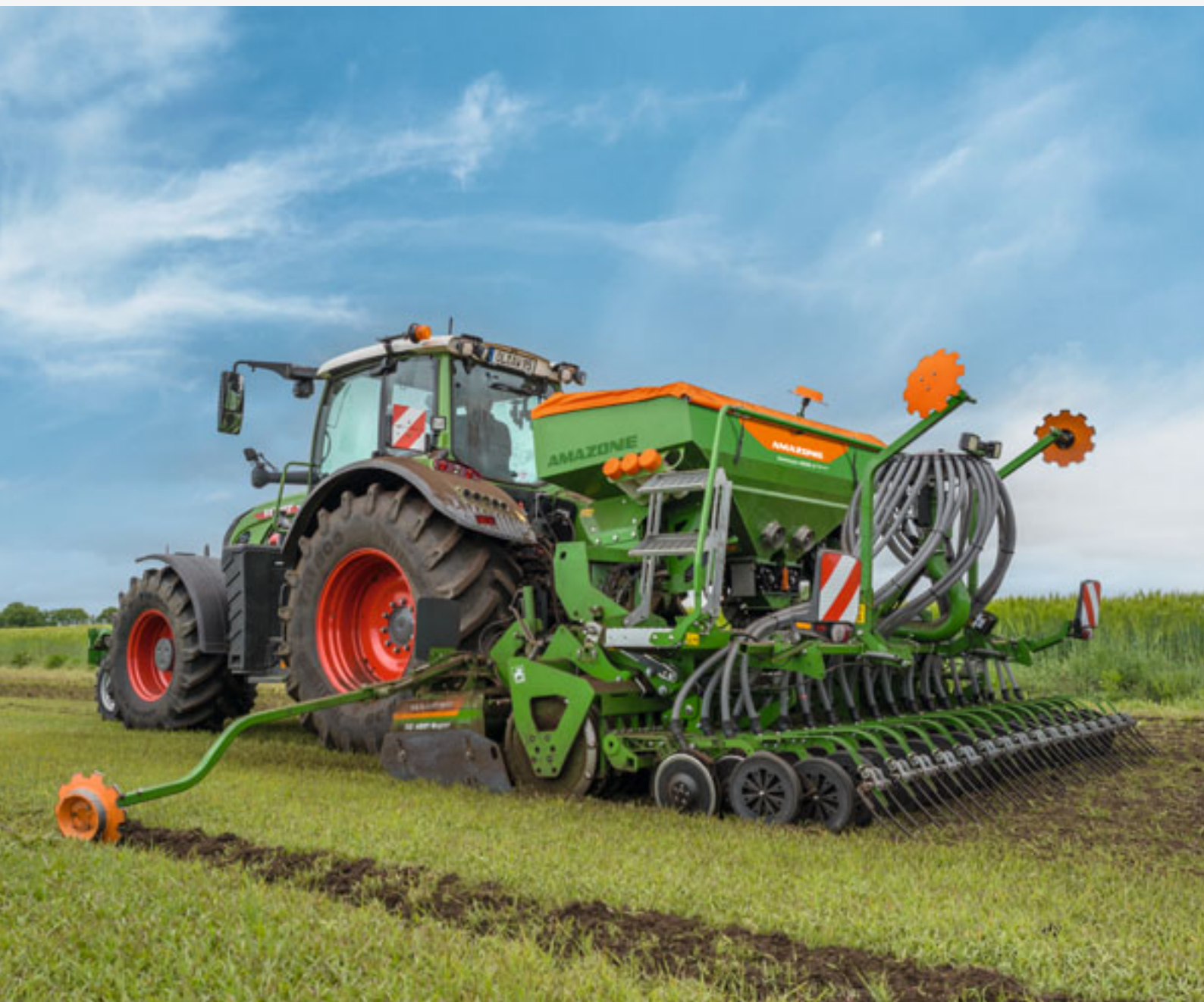
Centaya 4000-C Special mounted on a KG 4001 rotary cultivator. The soil is well mixed and loosened and the seed neatly placed in the sowing horizon via the TwinTeC double disc couler.
