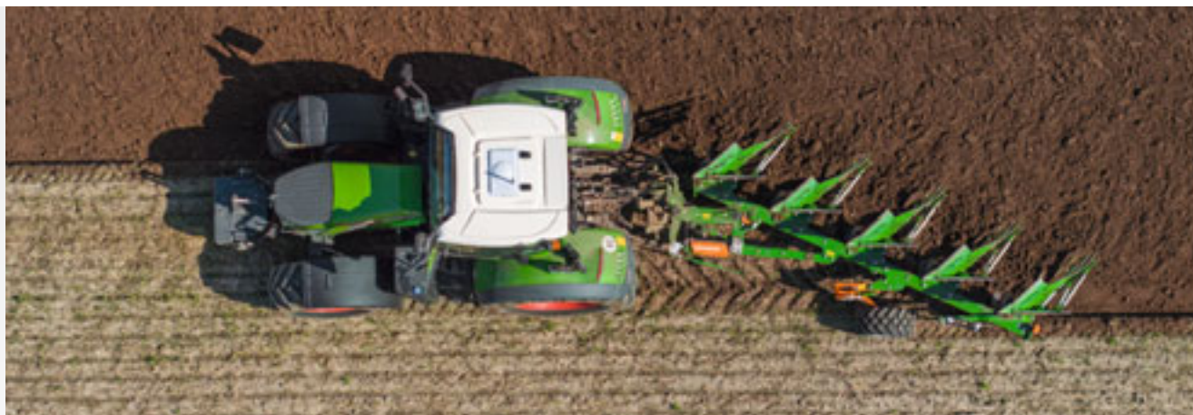
Optimum front furrow adjustment thanks to hydraulic front furrow adjustment
