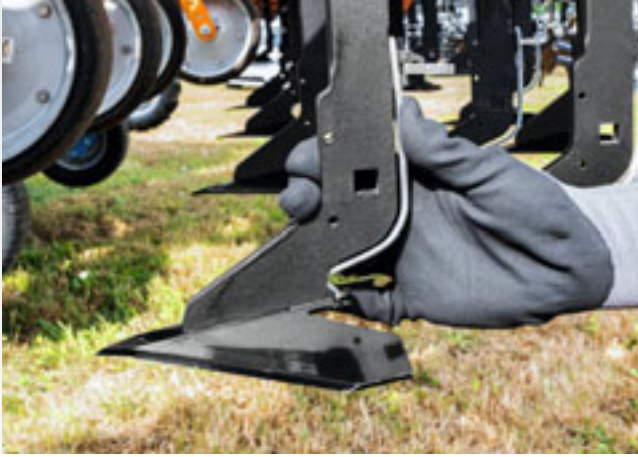
RapidoClip is the first tool-free quick-change system for hoe blades.
