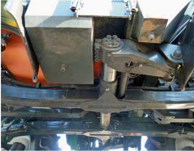
A beam on either side connects the front and rear wheels and pivots in the centre. It also allows the Pantera's track width to be altered.
