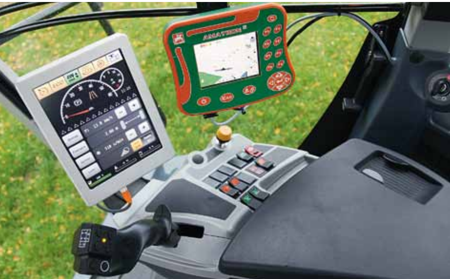
The large 10.4in Amadrive touchscreen looks after the skid unit functions, while Amatron 3 is responsible for the spraying equipment. Joystick is also used by Amazone fertiliser spreaders.
