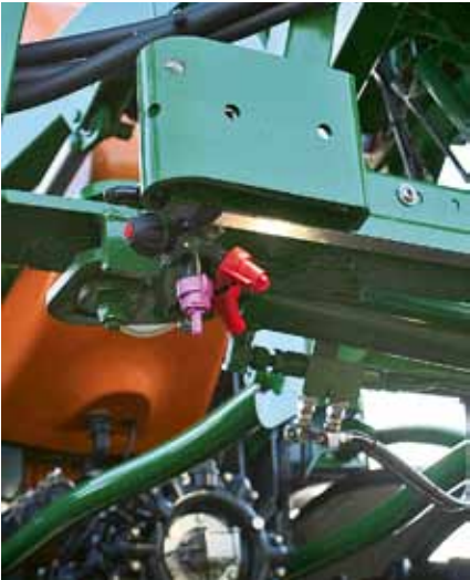
LED illumination of each nozzle is an extra-cost option and on a typical 30m boom lists at £3,000. This feature is also now available on Amazone's UX trailed sprayer models.
