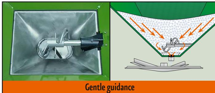
The AMAZONE Soft Ballistic System is incorporated into the slow-running agitators which are shaped in such a way that the fertiliser is taken from across the whole width of the hopper alleviating problems of the formation of a fertiliser funnel in the centre of the hopper and maintaining uniform spread pattern.
