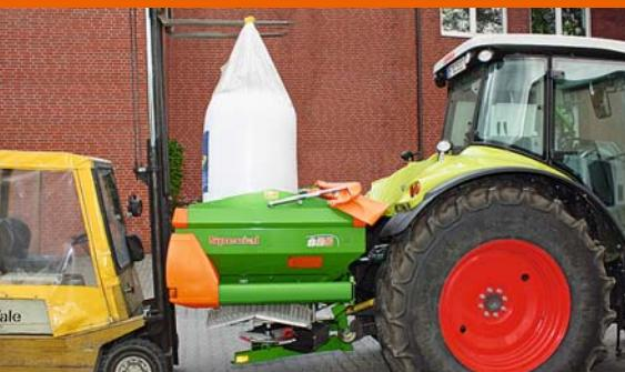
The hopper cover is simply swivelled open before filling. When closed it allows fertiliser spreading to continue, even during bad weather.
