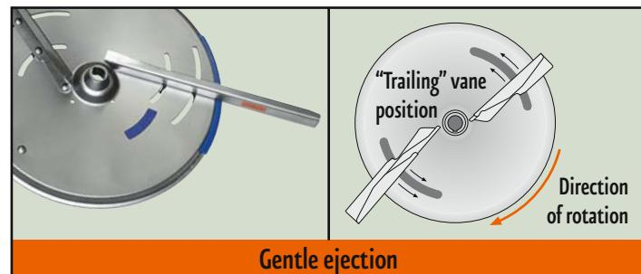
With the aid of the AMAZONE Soft Ballistic System the fertiliser is provided with the energy required for the optimum trajectory and a precise spread pattern.
