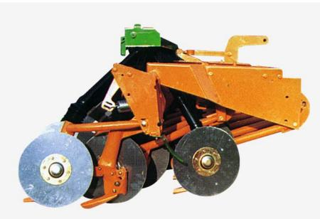
1980: First disc coulters with 3-row stagger for narrow sowing
