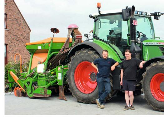
"No matter, whether heavy or light soils, whether conventional or mulch sowing – the machine is very flexible in operation", Sebastien and Gaëtan Delestrain summarise in their judgement of the AD-P. Additional strengths are for them, apart from the precise seed placement, above all also the simple handling and operation of the seed drill combination.
