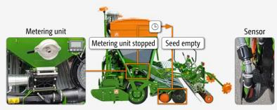
1. Split system: AutoPoint determines the conveying time
